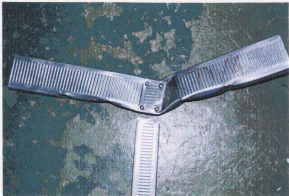
Photo 6.0 : After test – sample T1/4S (pulling test with 4 screws)
