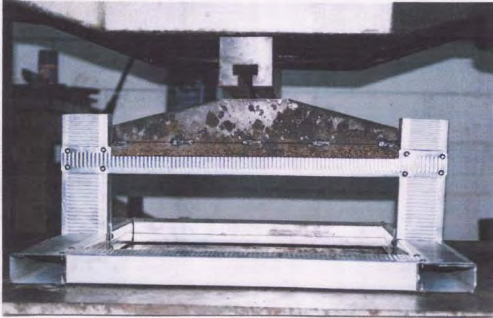
Photo 1.0 : Before test – sample S1/4S (compression test with 4 screws)
