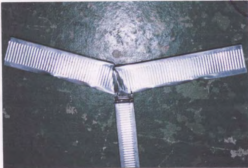
Photo 8.0 : After test – sample T1/2S (pulling test with 2 screws)
