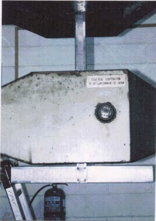
Photo 5.0 : Before test – sample T1/4S (pulling test with 4 screws)
