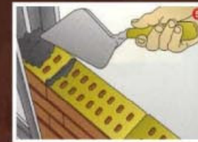
Brickwork is done by placing mortar into each gap between the brick and frame for each layer. This is to ensure that the frame is properly filled give rigidity and strength. Becoming an integral part of the wall and frame will add to the strength.
